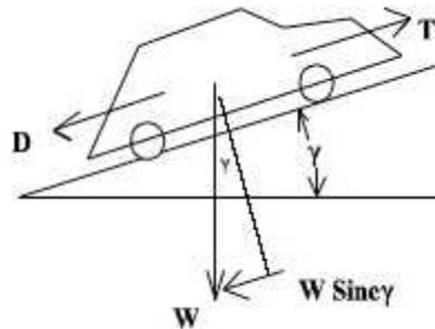
**Figure 1. Forces Along an Inclined Path**
